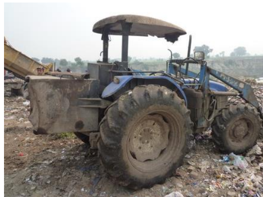
Photo 2.4.3 Landfill Tractor with Front Loading Bucket
