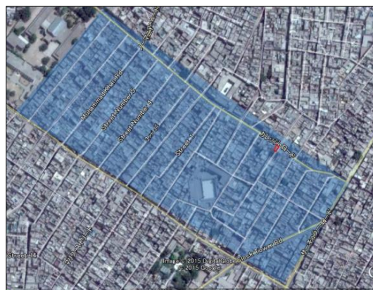
Figure 5.2.12 Sample Area for Estimation of Total Length of the Roads (Not to Scale)
