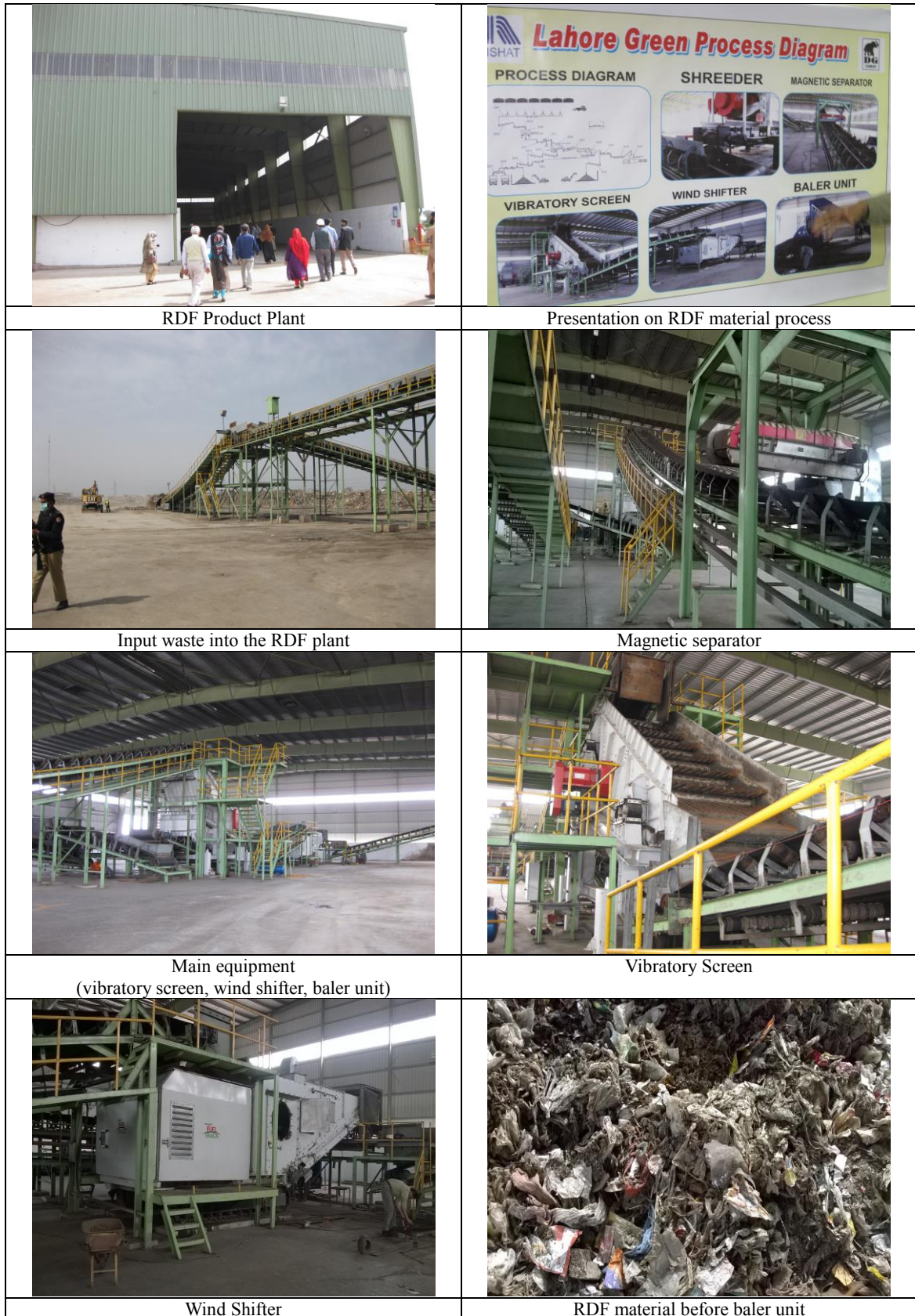
Photo 5.4.2 RDF Material Product under Operation of D.G. Khan Cement
