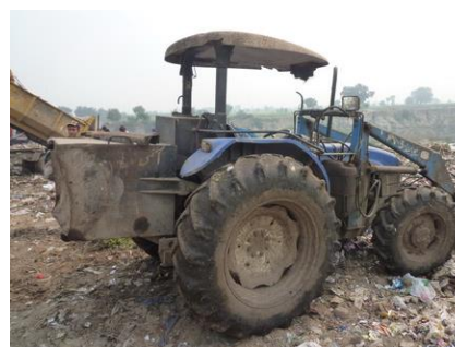
Photo 2.4.3 Landfill Tractor with Front Loading Bucket
