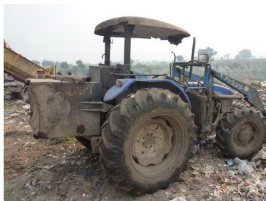
Photo C.2.3 Landfill Tractor with Front Loading Bucket
