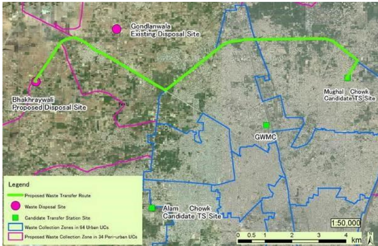
Figure B.4.3 Tentative Location of the Transfer Station at the Mughal Chowk Site
