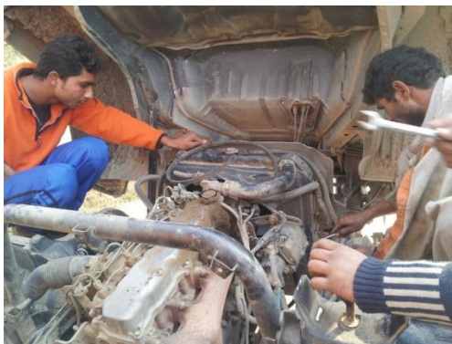
Figure 5: Repairing Fan Belt of Hino-11
