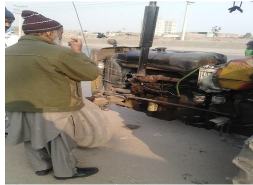
Figure 16: Engine Struck-out of TT-9774
